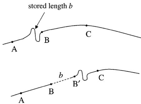
FIG. 1. The de Gennes–Edwards mechanism of translational motion of trapped chains via diffusion of “stored length defects”; the monomer at  $B$  moves by an amount  $b$  when the loop passes through it.
