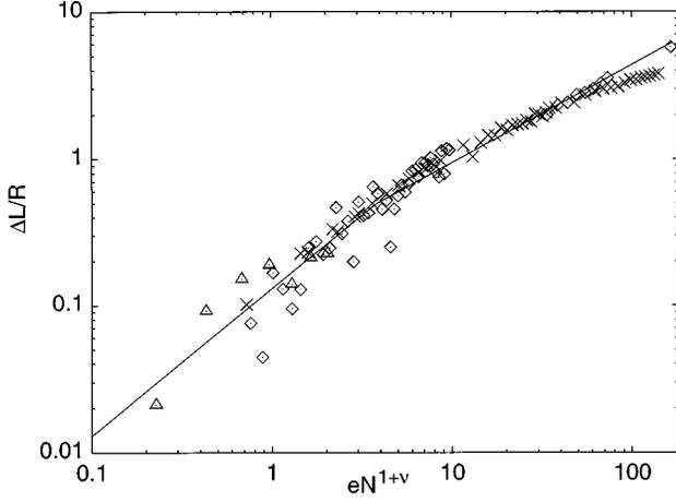
FIG. 4. Field-induced stretching of diblock PAs. Depicted is the relative stretching of the chain  $\Delta L/R$  as a function of  $eN^{\nu+1}$ ;  $e$  denotes the dimensionless field strength  $e = bqE/T$ . The straight lines correspond to the linear and to the Pincus regime (see text for details).
