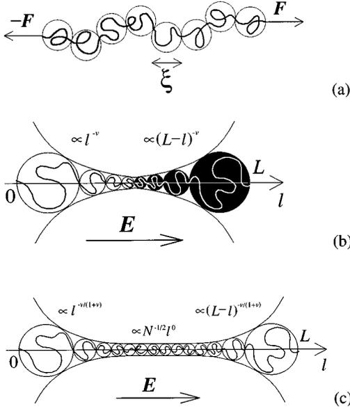
FIG. 3. (a) A polymer under traction (external force  $F$ ). The chain breaks up into a string of Pincus blobs of size  $\xi = T/F$ . (b) A diblock PA in an external electrical field (tug of war). The chain consists of a string of Pincus blobs of different sizes, constituting a double trumpet. (c) Equilibrium conformation of a random PA [using  $\bar{Q}_n$ , Eq. (16), as charge distribution; see text for details].
