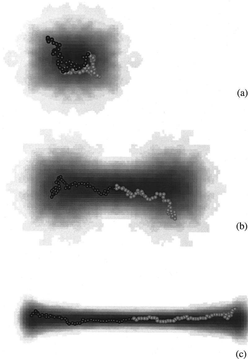
FIG. 5. Density plots of PAs at  $T=0.1$  in the (a) linear regime (slightly perturbed coil) with  $E=0.0005$ , (b) Pincus regime (double trumpet) with  $E=0.005$ , and (c) stem-and-flower regime with  $E=0.02$ . In each case we also present a snapshot of a particular realization.
