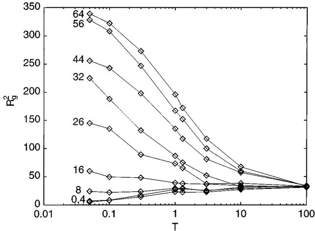
FIG. 1.  $R_g^2$  ( $b=1$ ) as a function of  $T$  for different values of the excess charge  $Q_{\text{tot}}$  for a 64-monomer chain. Each point is an average over ten independent runs at each temperature. The numbers near each curve denote  $Q_{\text{tot}}$  (in units of  $q$ ).
